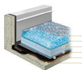
Blue Roof Assembly (typical stone ballasted blue roof depicted)
