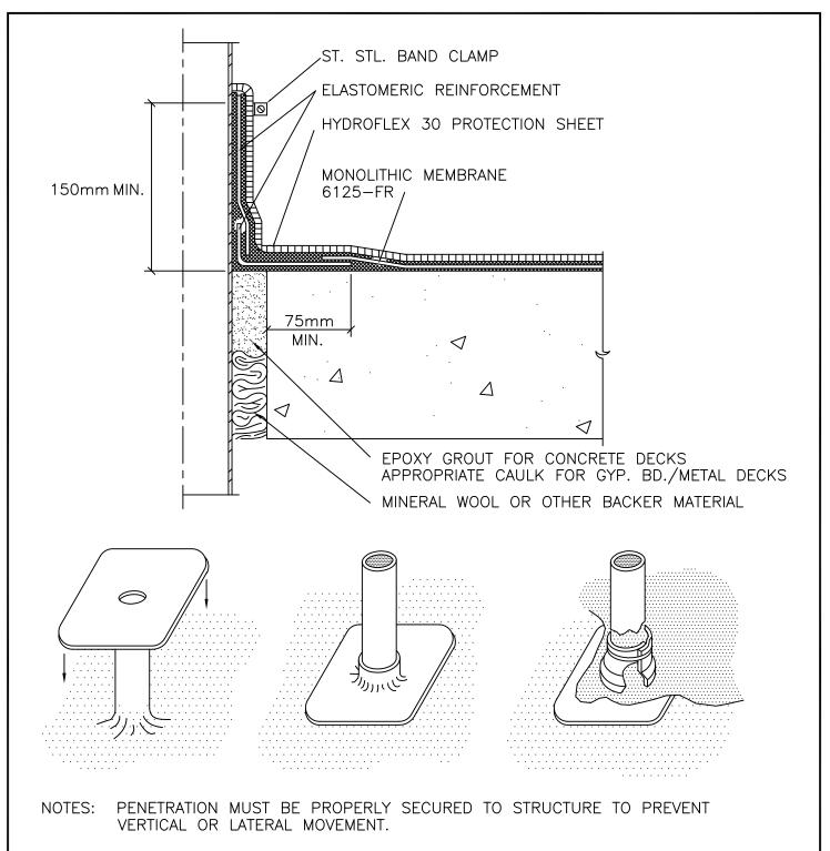
SOME PIPE MATERIALS (PVC, COPPER, BRASS) MAY REQUIRE ROUGHENING/SANDING, IN ADDITION TO PRIMING W/SURFACE CONDITIONER FOR PROPER ADHESION OF THE MM6125.
